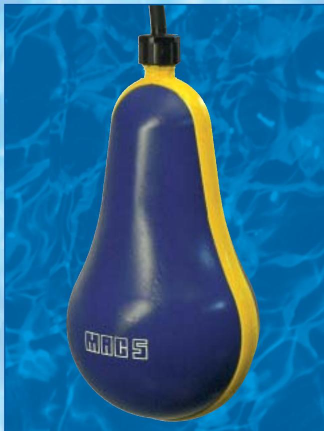
MAC 5 is an immersed tilting level regulator device. Its principal feature being its heavy body, which is also bulky and free of any irregularity, making it ideal for use in sewage water, in industrial waste water with suspended agglomerate residues and in tumultuous water. The polypropylene body is made with a double airtight chamber with high-pressure melted polypropylene re-injection sealing to ensure perfect sealing capacity against infiltrations.
